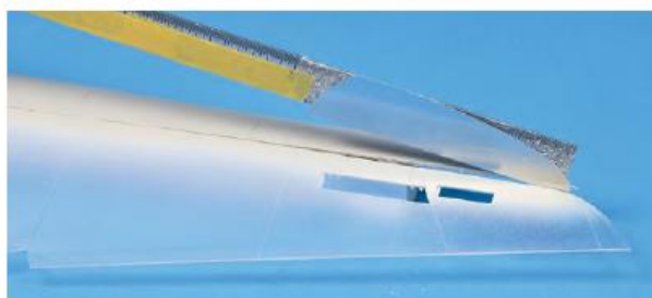
▲ The upper wing skins' leading edges were sawn along the existing panel line, with a PE saw blade taped to a steel ruler to provide rigidity. The wings were supported along the cut line, and multiple low-pressure passes avoid shattering the brittle clear plastic.
