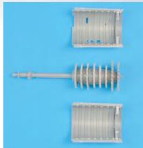
▲ The second engine's compressor blades were installed as spacers, but were cropped to avoid fouling the case...and just the front stator sections were used.
