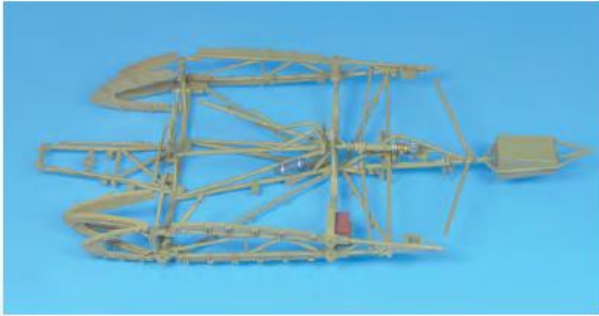
▲ With the basic structure completed, the framework was already surprisingly rigid, and the cutting mat jig was no longer needed...but many details still had to be added.
