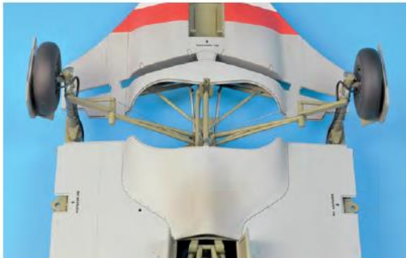
▲ The main gear actuation cables were added between the legs and extension ram, replicated by silver metallic thread. The latter was painted with thinned Citadel Chainmail to mute the shine.
