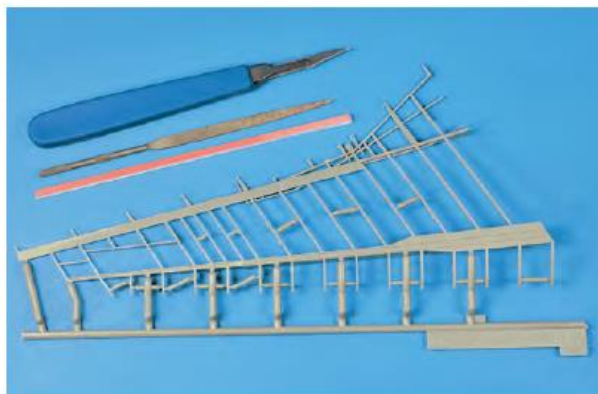
▲ Leaving the wing structure attached to the runners facilitated neatening, by protecting the leading edge ribs and stiffening the entire part. The gates were not cut until necessary.
