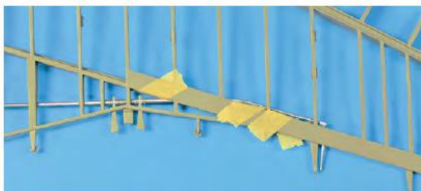
▲ In welcome contrast to the highly complex fuselage, each wing structure comprised just two parts, which needed careful detail painting. Here the torque tubes have been painted silver, with tape protecting adjacent areas from clumsy brushwork.
