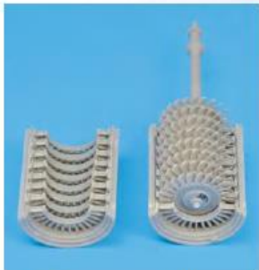
▲ The first engine was built with full compressor section detail. While impressive, it was quite fiddly and just the front rotor and stator were visible after assembly.
